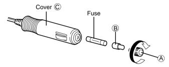
Insert the new fuse and part (B) into the cover (C), then turn part (A) in the direction of the arrow to fix it firmly.
